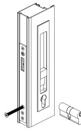
11. Place Strike plate cover onto base and adjust with screws for close fit.
