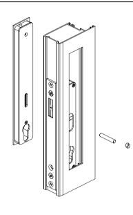
8. Push the euro cylinder lock through lock assembly, Tighten screw to lock cylinder in place.
