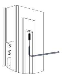
9. Align and Centre strike plate opposite the lock latch to suit engagement, measure the position of the strike plate from bottom of jamb. Mark and Drill holes for 10g screws to attach strike plate.
